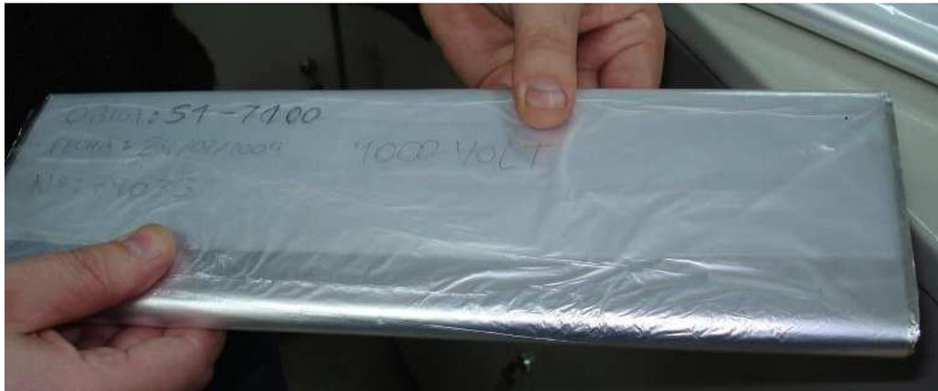
FIGURA 2.2 – MATERIAL INTERNO DO CAPACITOR PRONTO PARA TESTE
