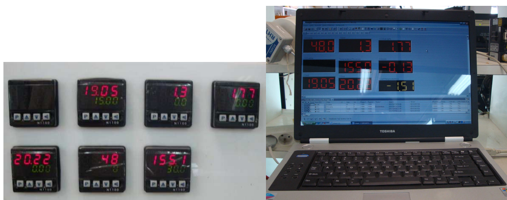
Figure 17. The Novus model N1100 controllers and the data acquisition by a personal computer with Laquis software.
