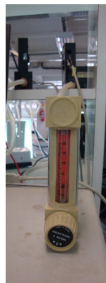
Figure 16. Rotameter used in CO 2 flow measurement in first plan. On the top at right there is the thermal dispersion mass flow sensor Aalborg GFM. On the top at left there is the other mass flow sensor (used for total flow measurement).
