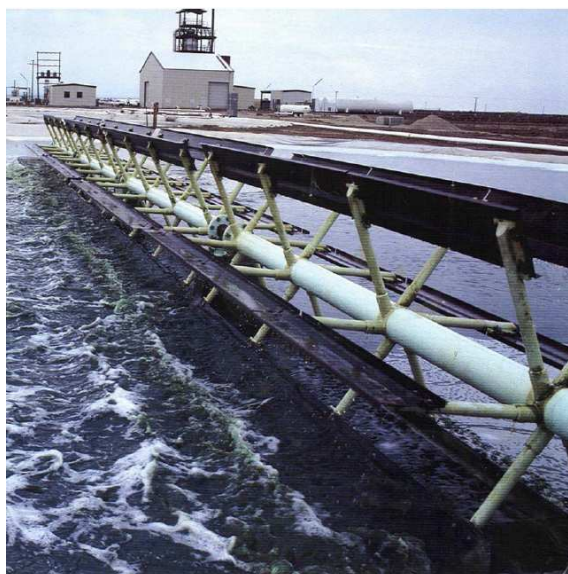
Figure 9. Paddle wheel mixing of raceway ponds in Earthrise Farms Inc.
