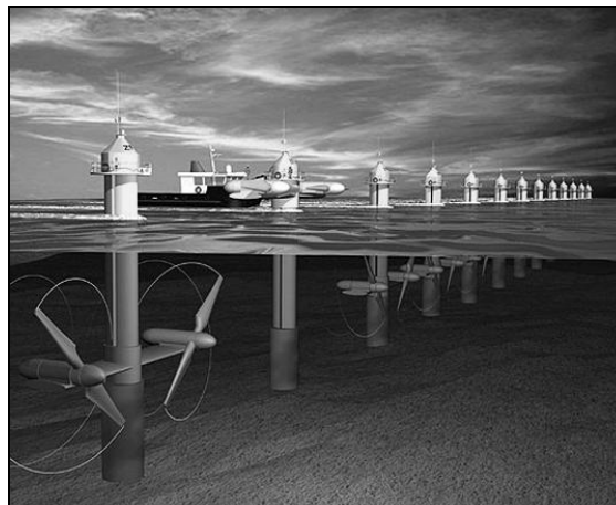
Figure 3-9: Scheme of some marine current turbines (ISET, 2005)
