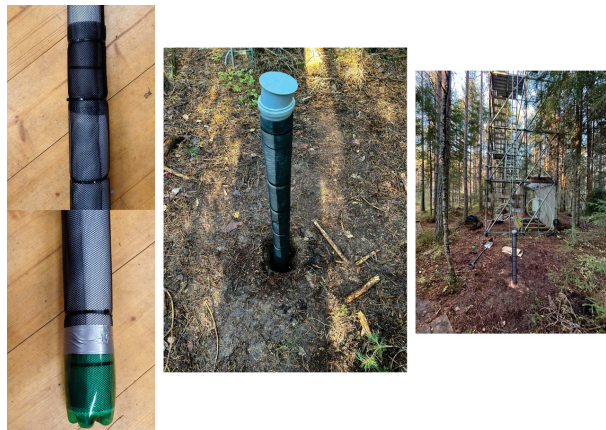
Figure 3.9: Water level sensor installed: on the left, its components and assembly procedure; in the center and on the right, the sensor installed near the SMEAR tower.
