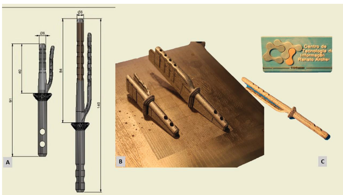
Figure 3 A: Final 3D prototyping of the patient's implants. B: Completion of the laser printing of the titanium implants. C: Presentation of the implant after removal of the holders. Carried out in partnership with the Renato Archer Information Technology Center – Campinas -SP.
