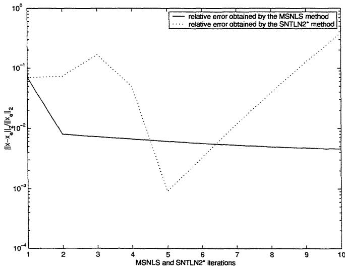
Figure 4.7: Comparison between both the MSNLS and SNTLN2\* methods with respect to  $x$  when  $b$  is perturbed by uniformly distributed random variables in the interval  $[-1.0\text{e-}8, 1.0\text{e-}8]$  and  $\gamma = 1.0\text{e-}1$ .
