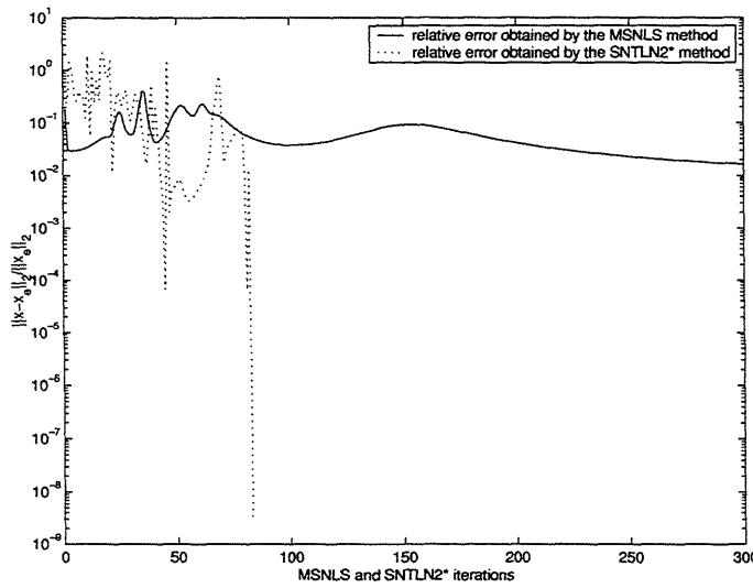
Figure 4.5: Convergence of both the MSNLS and SNTLN2\* methods with respect to  $x$  when  $b$  is perturbed by uniformly distributed random variables in the interval  $[-1.0\text{e-}8, 1.0\text{e-}8]$ ,  $\varepsilon = 1.0\text{e-}16$  and  $\gamma = 1.0\text{e-}1$ .
