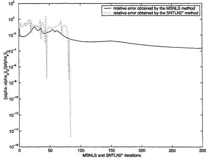
Figure 4.6: Convergence of both the MSNLS and SNTLN2\* methods with respect to  $\alpha$  when  $b$  is perturbed by uniformly distributed random variables in the interval  $[-1.0\text{e-}8, 1.0\text{e-}8]$ ,  $\varepsilon = 1.0\text{e-}16$  and  $\gamma = 1.0\text{e-}1$ .
