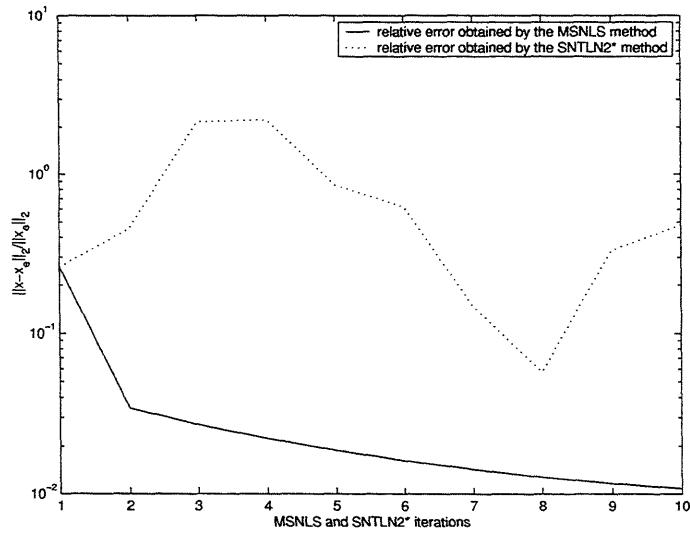
Figure 4.11: Comparison between both the MSNLS and SNTLN2\* methods with respect to  $x$  when  $b$  is perturbed by uniformly distributed random variables in the interval  $[\gamma, \gamma]$  and  $\gamma = 1.0e - 1$ .
