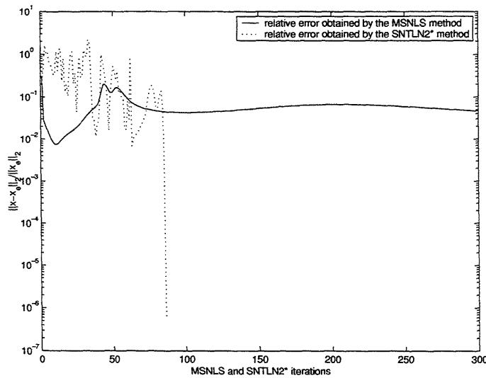
Figure 4.9: Convergence of both the MSNLS and SNTLN2\* methods with respect to  $x$  when  $b$  is perturbed by uniformly distributed random variables in the interval  $[\gamma, \gamma]$ ,  $\varepsilon = 1.0e-16$  and  $\gamma = 1.0e-1$ .
