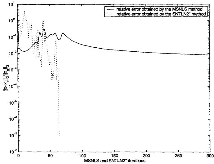
Figure 4.1: Convergence of both the MSNLS and SNTLN2\* methods with respect to  $x$  when  $b$  is unperturbed,  $\varepsilon = 1.0e - 16$  and  $\gamma = 1.0e - 1$ .
