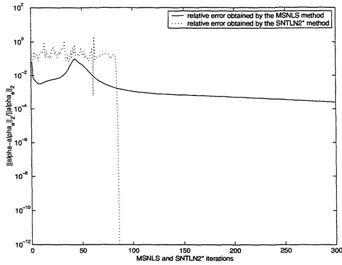
Figure 4.10: Convergence of both the MSNLS and SNTLN2\* methods with respect to  $\alpha$  when  $b$  is perturbed by uniformly distributed random variables in the interval  $[\gamma, \gamma]$ ,  $\varepsilon = 1.0e-16$  and  $\gamma = 1.0e-1$ .
