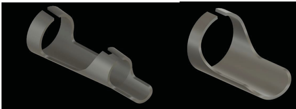
Figure 2. Representative examples of the spacer prototype made by the Software CAD Fusion 360, for both tonometers TD8 (left) and TVV (right).
