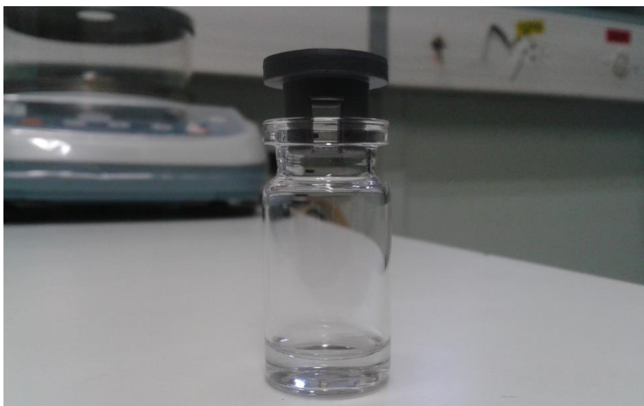
Figure 3.5: 7.5 mL glass vial filled with 1 mL and partially closed with a rubber stopper.
