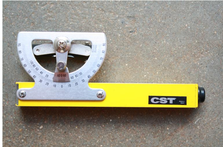
FIGURA 8 – CLINÔMETRO TIPO ABNEY, MARCA CST
