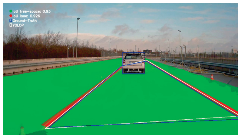
Figure 38 – Lane polygon YOLOP/Ground-truth.
