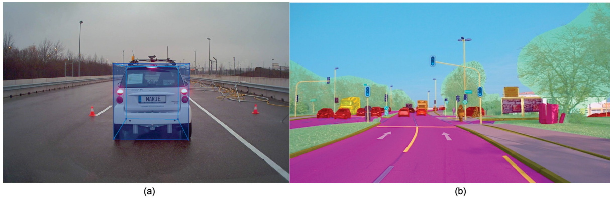
Caption: (a) 3D bounding box (b) Semantic segmentation. Source: (a) (NETO et al., 2023) (b) (GEYER et al., 2020).
