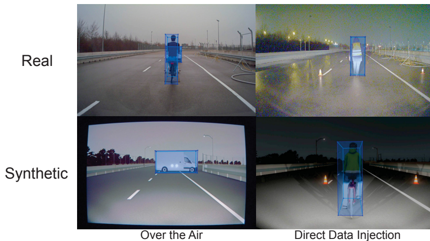
Figure 43 – Projected cuboid onto objects.
