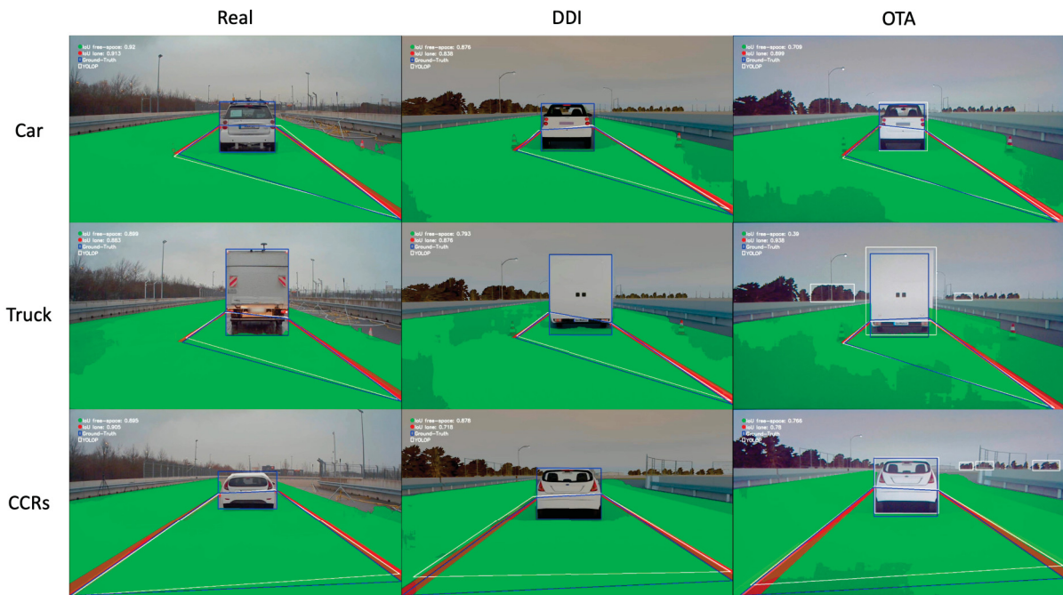
Figure 50 – YOLOP detections with ground-truth.
