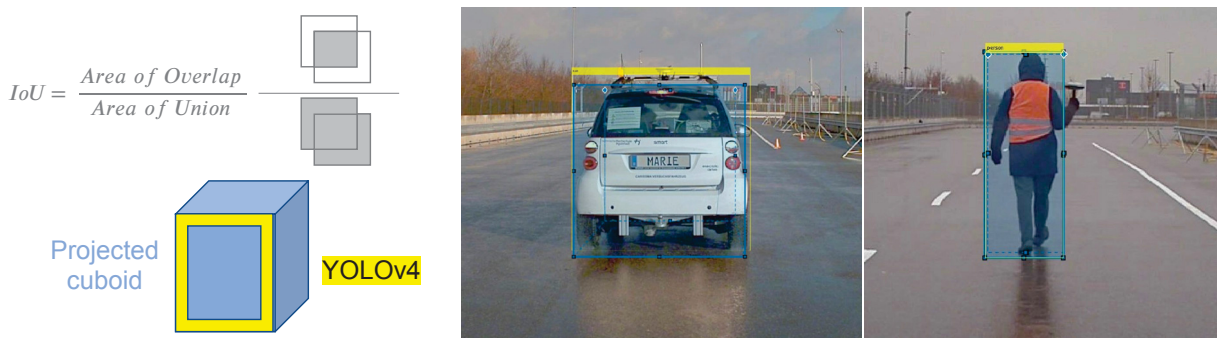
Figure 34 – IoU between projected cuboid and YOLOv4 detection.
