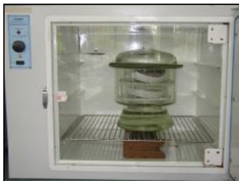
Figure 1. Sieves containing substrate incubated in humid chamber at 28°C
