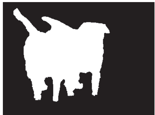
(b) Example of a ground-truth mask, with the pixels corresponding to the salient objects (the dogs) in white and the pixels corresponding to the background (the grass) in black.
