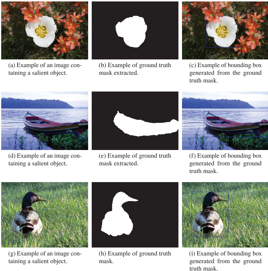
Figura 5.1: Examples of salient objects extracted from the MSRA10K dataset. Figures 5.1a, 5.1d, and 5.1g presents examples of images containing salient objects, Figures 5.1b, 5.1e, and 5.1h presents examples of the ground truth mask, and Figures 5.1c, 5.1f and 5.1i presents an example of bounding boxes generated from the ground truth masks. Source: Cheng et al. (2015).
