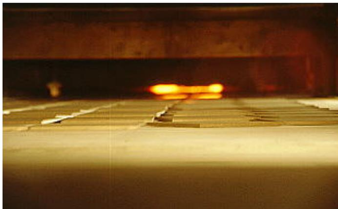
FIGURA 2.12 – FORNO A ROLO MONOCANAL <sup>[25]</sup>.
