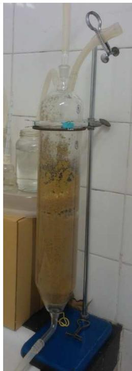
FIGURA 23 – PRODUÇÃO DE MANANASE POR FESS COM CS (15%, m/v) E *A. niger* NRRL 328 EM BIORREATOR BCR
