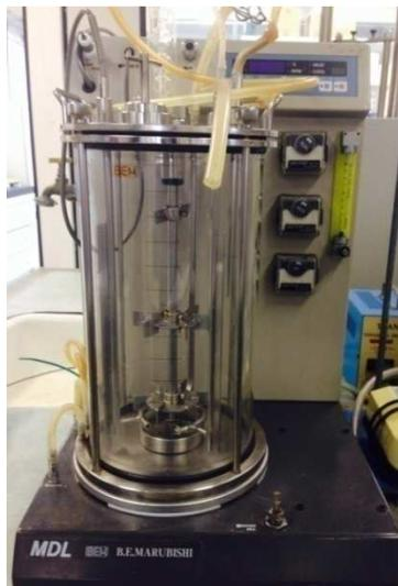
FIGURA 9 – BIORREATOR MODELO MDL 750 (B. E. MARUBISHI THAILAND Co. Ltda.), UTILIZADO PARA PRODUÇÃO DE MANANASE POR FESS
