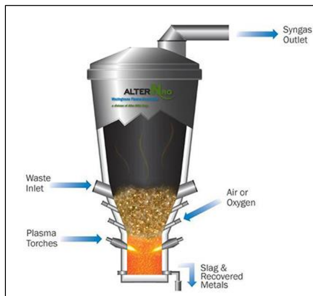
Figure 16 – Schematic of a Plasma gasifier. Source: AlterNRG.
