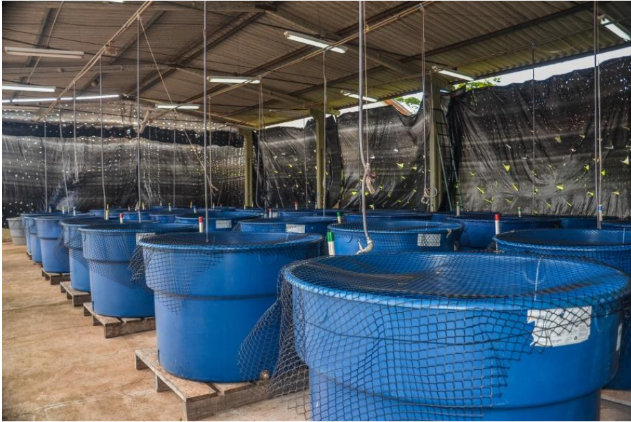
Figure A19. Curtains closed during direct sunlight hours and mesocosms protected with 2.5 cm mesh.
