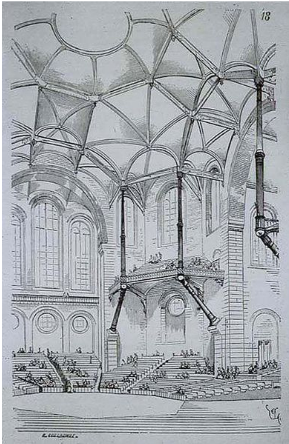
FIGURA VI Design for a Concert Hall, 1864 Expressing Gothic Structural principles in Stone, Brick and Cast Iron.
