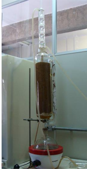
FIGURA 6 - APARELHO DE SOXHLET
