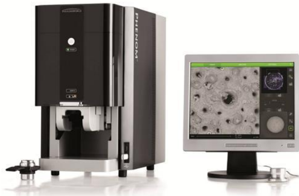
Figura 18 – MEV de bancada Phenom (LITS)
