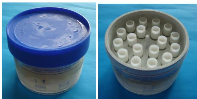
FIGURA 6: Aparato Mr. Frosty® Freezing Container (Nalgene)
