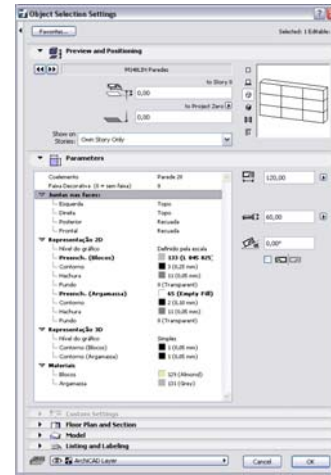
Fig. 4: Settings panel of a parametric wall object.
